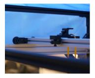
**Figure 2.** Horizontal sliders move in the XY plane as the user moves their arms to mimic a swimming gesture. The sliders are attached to resistance bands (in yellow), which are attached to user's arms and legs to simulate drag forces. Neoprene sleeve attachments are used to distribute forces uniformly on the user's limbs.
