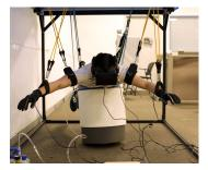
**Figure 1.** Amphibian is an immersive virtual reality system that enables people to experience ocean SCUBA diving in a convenient terrestrial setting. Images above show (a) the Prototype II suspension frame and (b) a user suspended in the harness, as needed for experiencing Amphibian.
