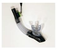
**Figure 4.** Mouth piece with Sensirion gas flow sensor [20] that measures the amount of air inhaled and exhaled by the user. lessons learned during the preliminary deployment of Prototype I.
