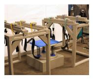
**Figure 7.** Amphibian Prototype I consisting of a smaller wooden rig and a spring torso rest.
