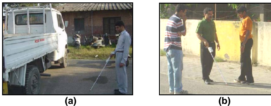
Figure 3: Smart Cane utility (a) detection of the raised side of a truck and (c) finding a clear path without colliding with randomly positioned observers.
