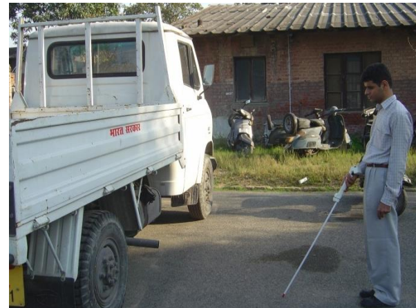
Raised obstacle detected 3m away 7
